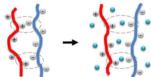
**Figure 4.** Simplified mechanism of how the water uptake affects the interactions between PEI and PAA. The effect of water can significantly disrupt the cross-linked network and activate the motion of the whole polymer chains. The red line and the blue line respectively represent PEI and PAA; the blue dots correspond to the water molecules within the film.
