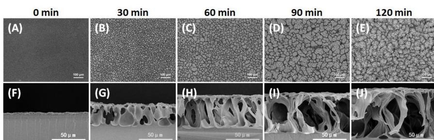
**Figure 1.** Acid-induced structural evolution of  $(PEI/PAA)_{15}$  films over time. Optical microscopy images (A-E) and SEM cross-sectional images (F-J) of the PEM films after immersion in pH 2.9 for various times. Freeze-drying was performed to remove water before SEM examination. The default immersion time was set to 60 min in the study of drug delivery.
