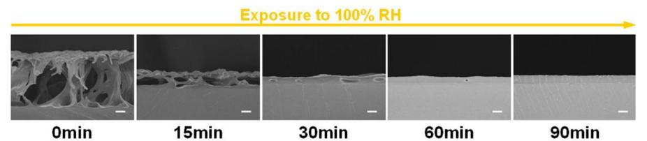
**Figure 3.** SEM cross-sectional images of the healing process of the microporous PEM film. All of the inset scale bars represent 10  $\mu\text{m}$ .
