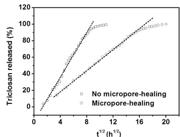
**Figure 5.** Release profiles of triclosan from the drug-loaded PEM films without (A) and with (B) micropore-healing. The linear relationships between the drug releasing percent and the square root of the releasing time at the early stage indicated that the drug releases followed a Fickian diffusion mechanism. The closure of those microporous structures is favorable for the sustained release of drugs.
