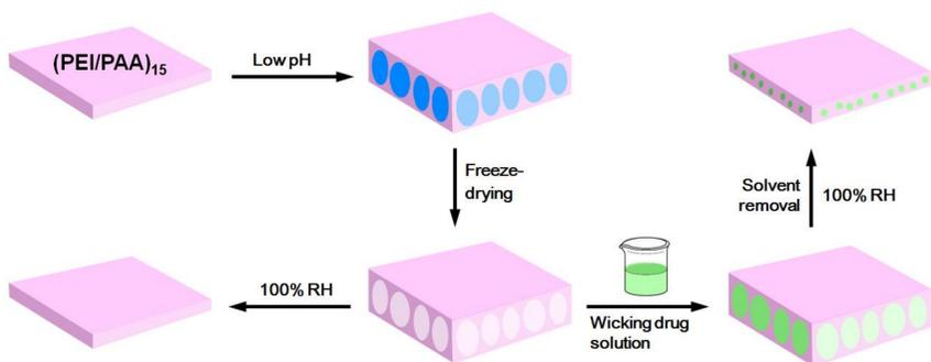
**Scheme 1.** Fabrication of dynamic polyelectrolyte multilayer (PEM) film with self-healing microporous structures and integration of hydrophobic drug into the film.
