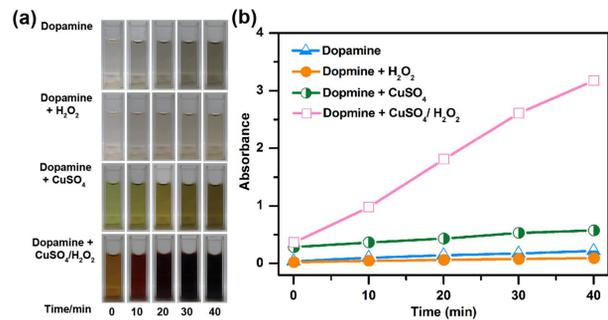
**Figure 1.** a) Photographs of original dopamine solutions with various additives (CuSO<sub>4</sub>: 5 mM; H<sub>2</sub>O<sub>2</sub>: 19.6 mM) at different time points. b) Time-dependence of absorbance at 420 nm for various diluted dopamine solutions.
