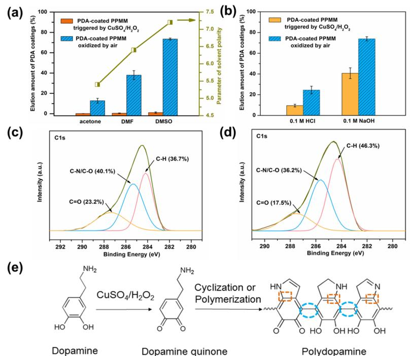
**Figure 3.** a) and b) Elution amount of the PDA-coated PPMMs immersed in different solutions. c) High-resolution XPS spectra of PDA coatings on silicon wafer triggered by CuSO<sub>4</sub>/H<sub>2</sub>O<sub>2</sub> for 40 min. d) High-resolution XPS spectra of PDA coatings on silicon wafer oxidized by air for 12 h. e) Illustration of the reduction of C-H during the process of dopamine polymerization.
