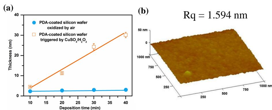
**Figure 2.** a) Time-dependence of thickness for the PDA coatings deposited on silicon wafers, as determined by ellipsometry. b) AFM images of the PDA-coated silicon wafer triggered by CuSO<sub>4</sub>/H<sub>2</sub>O<sub>2</sub> for 40 min.
