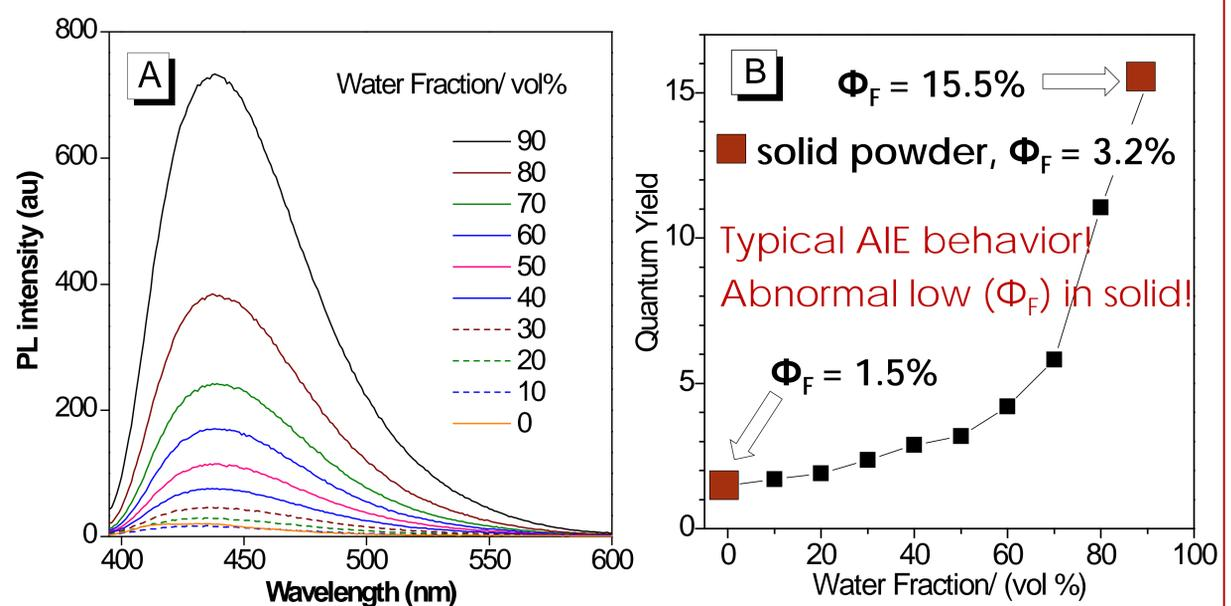
**Fig. 3.** (A) Photoluminescence (PL,  $\lambda_{ex} = 375$  nm) spectra of Box in DMSO/H<sub>2</sub>O mixtures with different H<sub>2</sub>O fractions ( $f_w$ ). (B) Changes in PL quantum yield ( $\Phi_F$ ) in DMSO/H<sub>2</sub>O mixtures. [Box] = 10  $\mu$ M.
